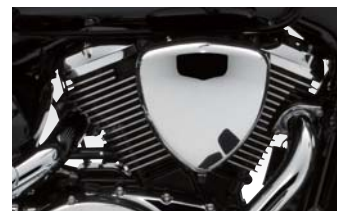
Liquid-cooled 45-degree V-Twin engine
